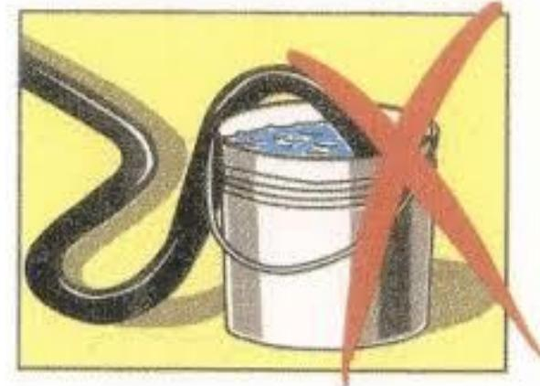
**DO NOT use spray attachments without a backflow prevention device. The chemicals used on your lawn are toxic and can be fatal if ingested.**
